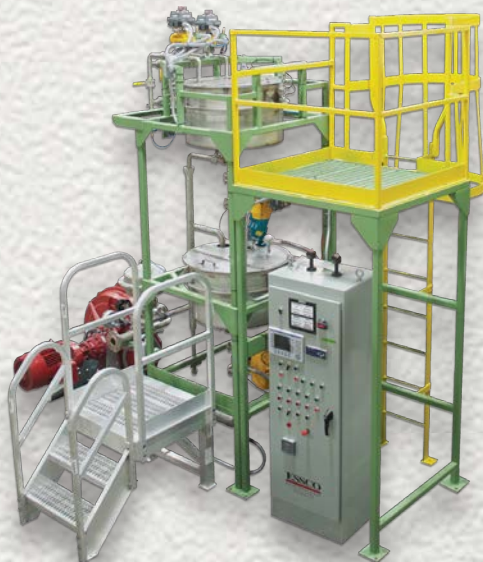
Extremely precise water weigh system utilizing ESSCO's control capabilities and Tencarva Fabrication expertise
